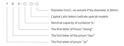
Example 1:YDS-30 refer to a liquid nitrogen container with capacity of 30L and diameter of 50mm.
